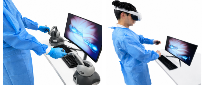
Fig. 6. Operator-driven SurgCast with a physical 6-DoF surgical master device (left) and VR controllers (right) as sources of prospective action commands. Displays show the generated surgical view; action-dependent outputs are compared in Fig. 7.
